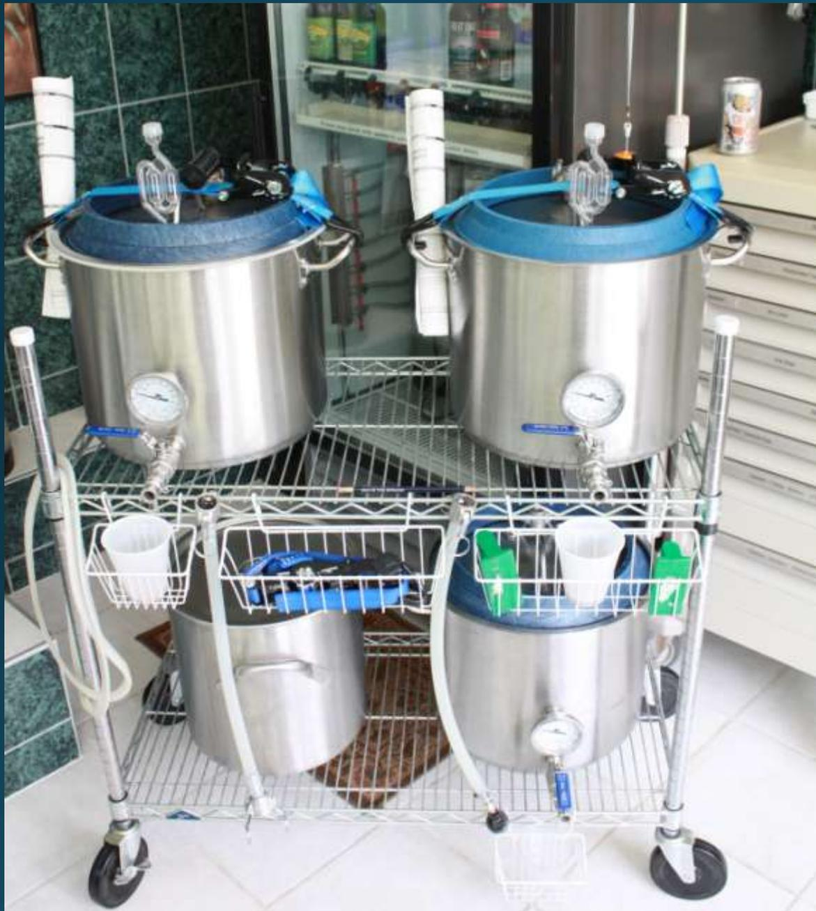
Mark switched to custom built stainless fermenters, basically modified 8-gallon kettles. Drilled lid to add airlock/blowoff and a camlock port welded in to allow yeast pitching and transfer between vessels. A silicon gasket, ratchet strap and modified dog food bowl round out the modifications. These are easy to clean and for me, to move and double as mash tuns.
