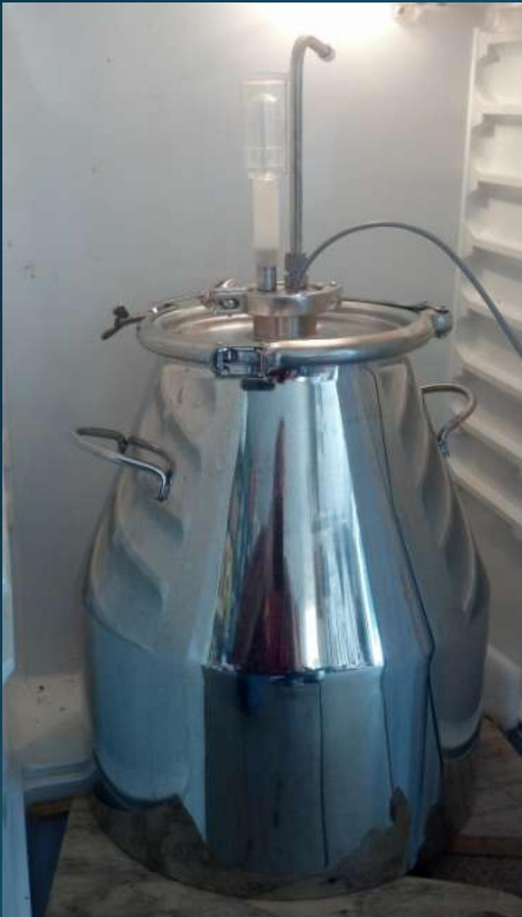
Jim Gress uses these hybrid stainless fermenters. They are 8-gallon modified "milk-can" distilling kettles from [Brewhaus.com](http://Brewhaus.com) that have been fitted with a Sanke Fermenter Conversion Kit from [Brewershardware.com](http://Brewershardware.com) that features integrated thermowell, stainless racking cane and blow-off port. These can be pressurized to "push-rack" with CO<sub>2</sub>. The kettles are also available in a 15-gallon size.
